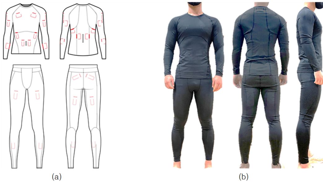
Fig. 10. Prototype of EMG measuring device-combined clothing; (a) flat design, (b) real fitting.
