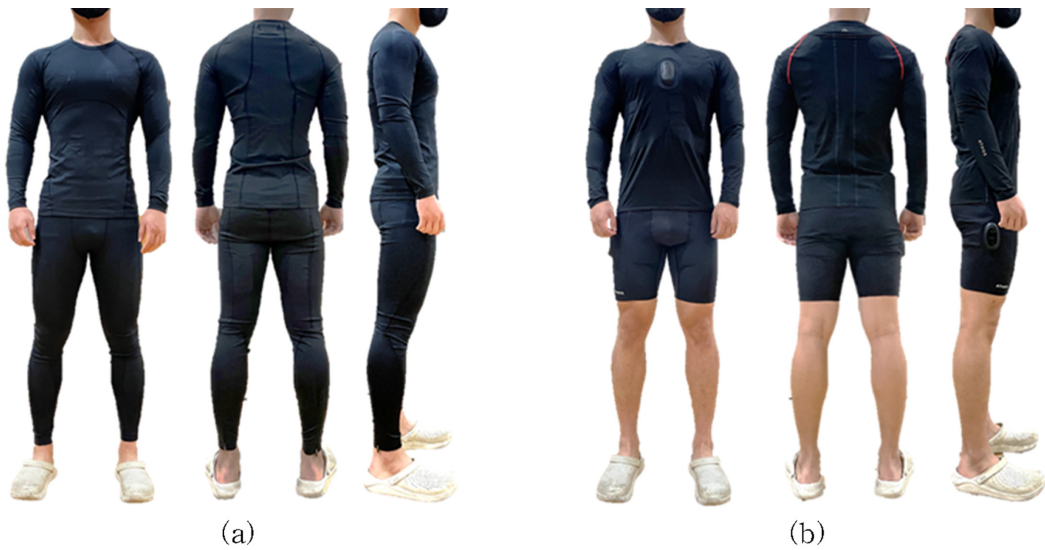
Fig. 8. EMG measuring clothing; (a) development of EMG measuring device-combined clothing, (b) commercial EMG measuring clothing.
