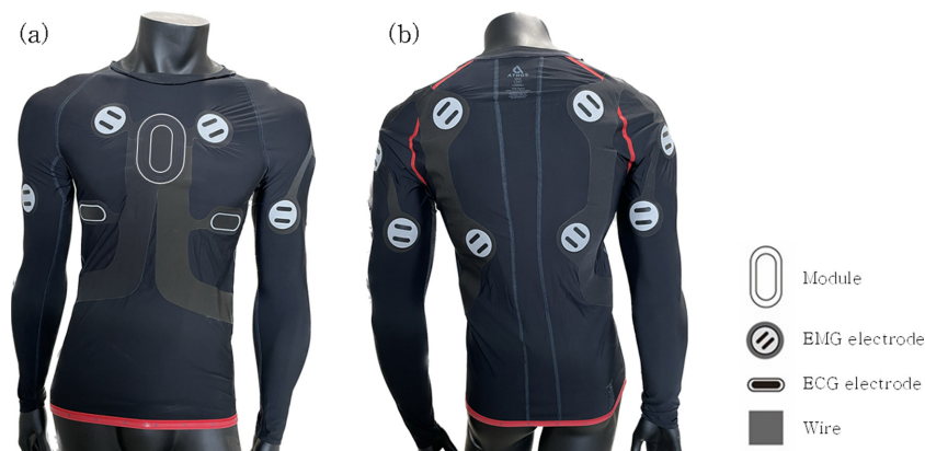
Fig. 2. Example of the structure of EMG measuring clothing(inside of the Athos shirt); (a) front, (b) back.
