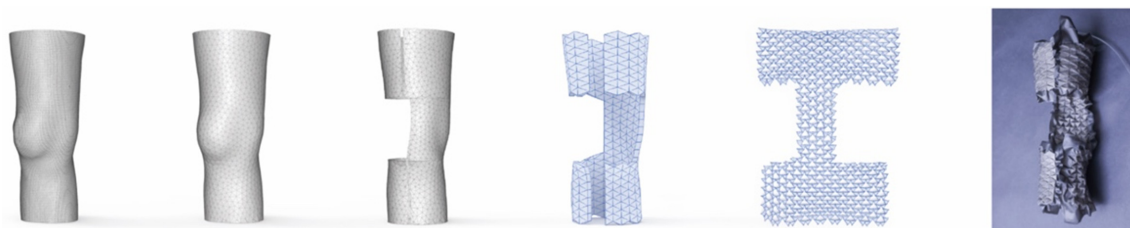
Fig. 12 Pneumatic Auxetics provides support when deflated and can be adapted to the scanned surface of the patient's knee(Eguchi et al., 2022).
