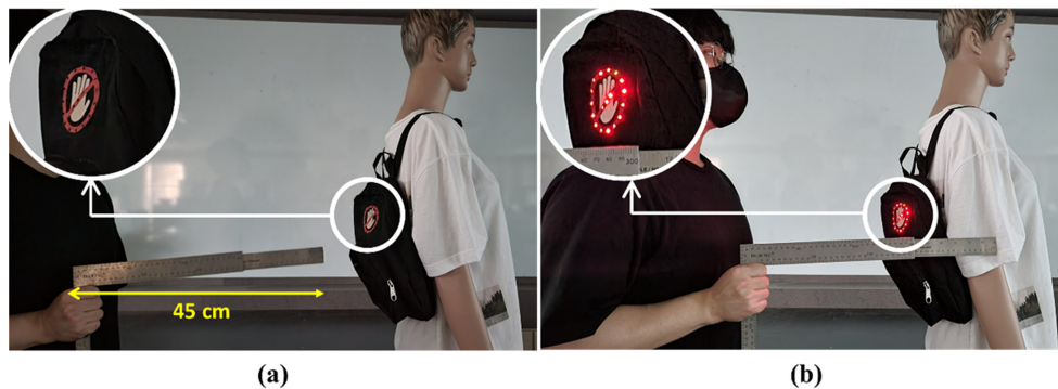
Fig. 9. Photograph of operated smart backpack system with a person within 45 cm range.
